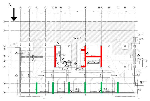
Figure 4: Foundation Plan (Level PO) Showing Shear Walls (Source: Cagley & Assoc. Drawing S-200)
