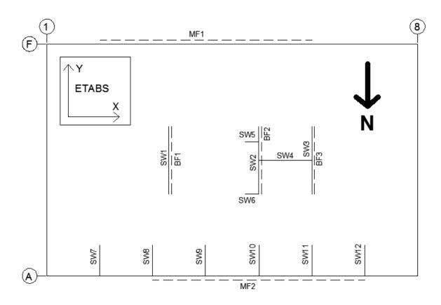
Figure 18: Labeling of Lateral System Elements (Source: Chavanic)
